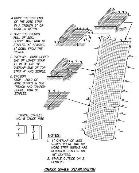
JUTE NETTING TEMPORARY SLOPE AND SWALE STABILIZATION
