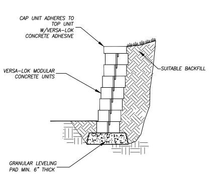
1. MATCH TYPE AND COLOR OF EXISTING VERSA-LOK WALL. 2. DESIGN AND INSTALLATION TO BE PREAPPROVED BY THE MANUFACTURER'S ENGINEER.
