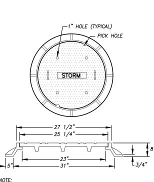
CONTRACTOR IS TO CONFIRM THE DIMENSIONS OF THE EXIST. STRUCTURE PRIOR TO ORDERING THE MANHOLE FRAME AND COVER.
